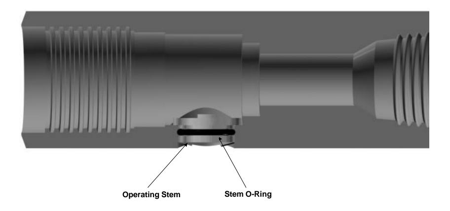
11. Apply grease to the seat, o-ring, and seal ring. Install o-ring and Teflon seal ring on the seat.
